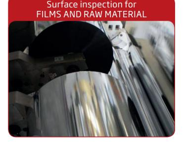
reduction. When a defect is found, the operator is alerted and the type of defect is logged in order to provide a detailed report for each roll.
