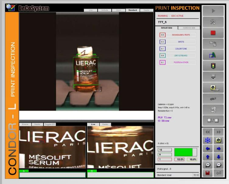
Screenshot of the GUI that shows the control mode and the acquired image from the line camera.
