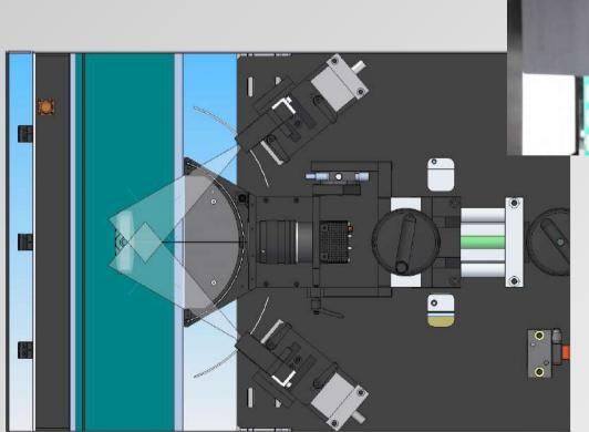
The line camera perform the acquisition while the bottle is moving in front of the camera.
