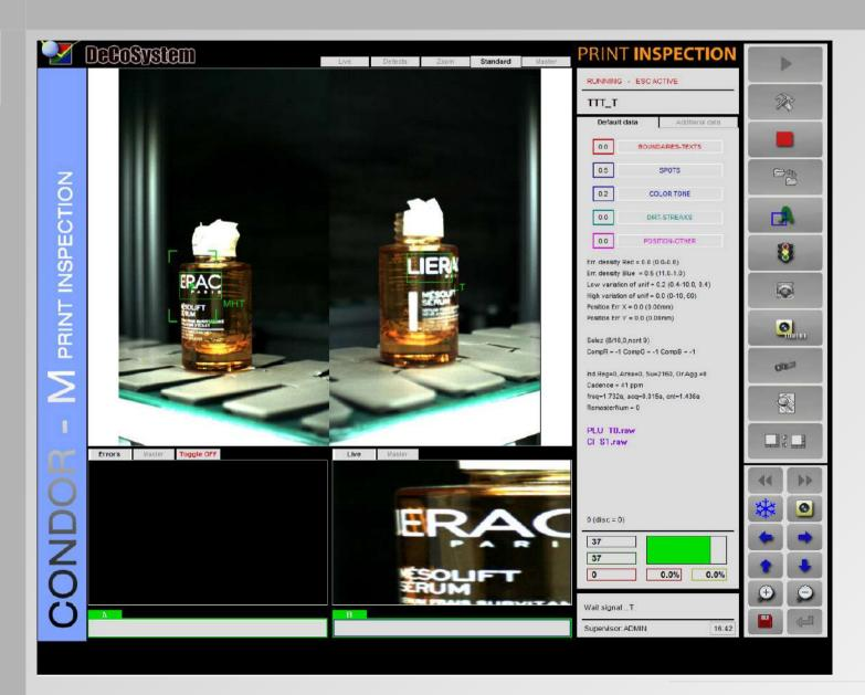
Screenshot of the GUI that shows the control mode and the acquired image from the matrix cameras.
